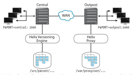
In this configuration, file revisions requested by users at a remote development site are fetched first from a shared server (**p4d** running on Central) and transferred over a relatively slow WAN. Subsequent requests for that same revision, however, are delivered from the Helix Proxy, (**p4p** running on Outpost), over the remote development site's LAN; this architecture reduces both network traffic across the WAN and CPU load on the shared server.
