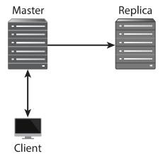
When you create the replica, you specify which server it should get its data from. The replica then periodically updates itself by copying files and metadata from the master. If the master fails, all you need do is reconfigure the replica to be the new master and then reconnect clients to communicate with it.
