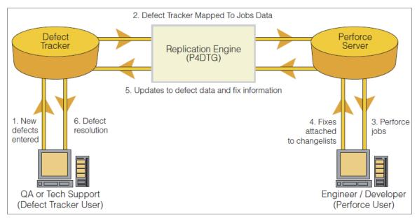
The following diagram provides an overview of the gateway components and shows how data is transferred.
